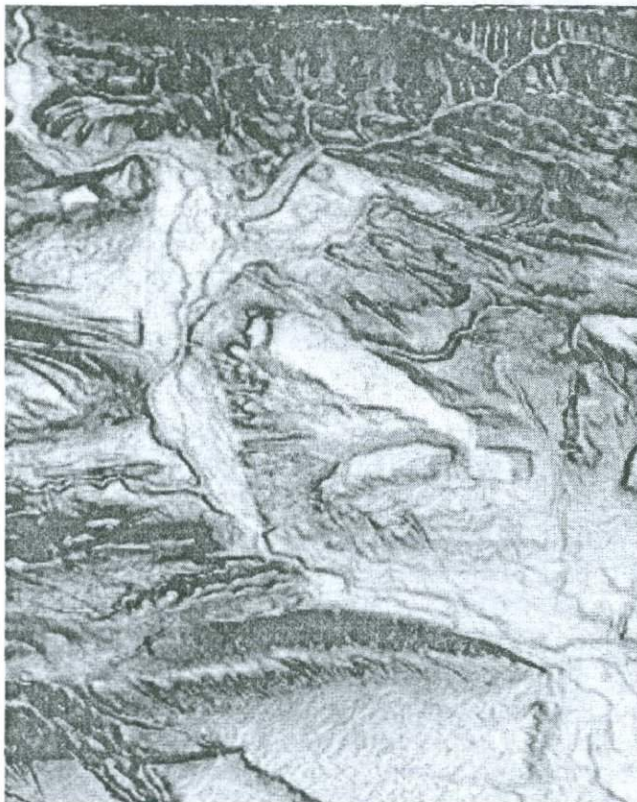
Fig. 2. SRTM – Shuttle Radar Topography Mission. Spatial Resolution = 90 v. Wavelength = 5.6 and 3.1 sm. Data: 2000, 17.02.
