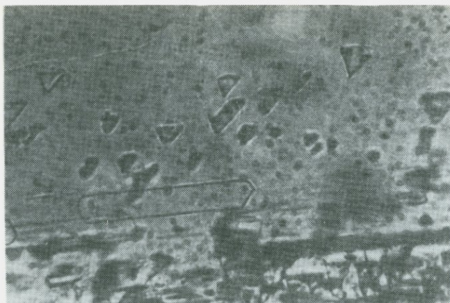
Fig. 8. Monophase liquid inclusions with the shape of negative crystal and triangular monophase liquid inclusions in secondary gypsum. Sample G-02 from a certain antimony ore deposit in China, x 450
