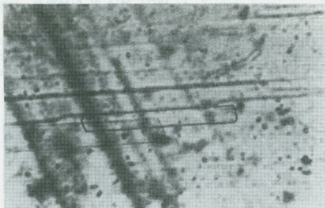
Fig. 9. Monophase liquid inclusion with the shape of negative crystal in gypsum. It is parallel to one set of cleavages. Sample G-05 from a certain antimony ore deposit in China, x 450
